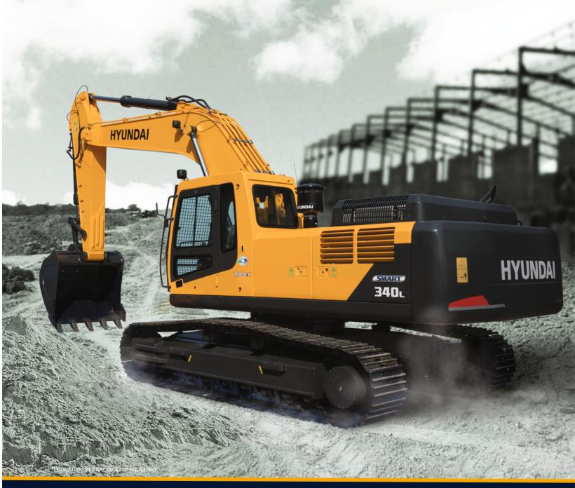
Engine Rated Power 276 HP (206kw) @ 1900rpm
